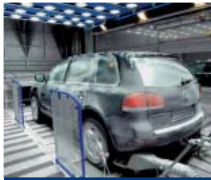
Altitude Temperature Test Chamber with 4-wheel-drive Dynamometer and Sunlight Simulation
