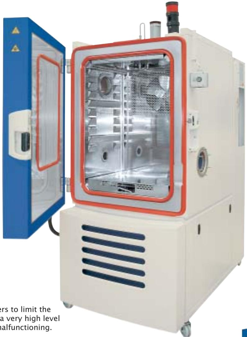
Additional STB safety temperature limiters to limit the maximum test chamber temperature at a very high level of reliability even if the test cabinet is malfunctioning.
